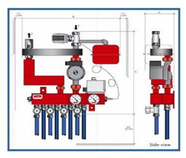
ball valve with flow meter and connections for the heating tube, high limit thermostat, condensation sensor and 24V thermal actuators.
